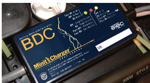
BDC Battery Module
