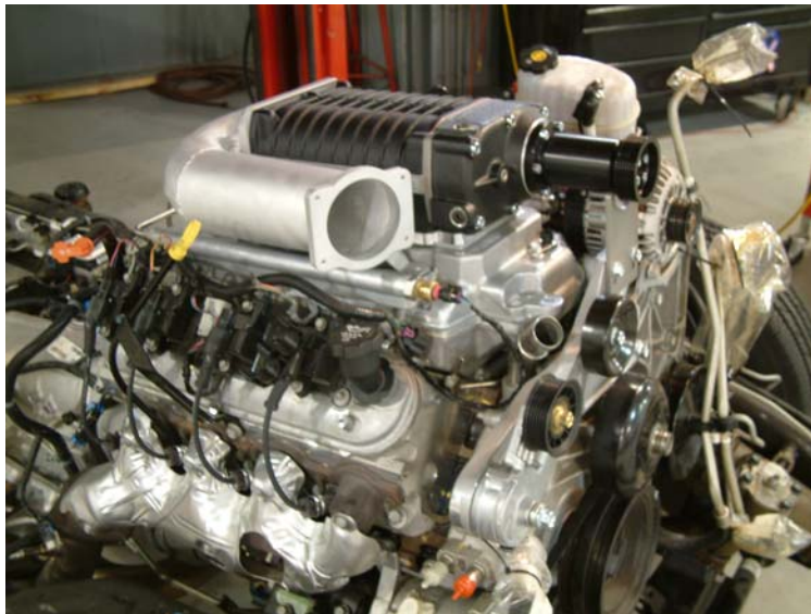
Vortec 6.0L V8 with Supercharger and Intercooler Installed
