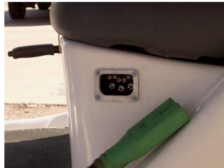
Figure 4.4 Charge Receptacle Assembly – Mounted under the Driver's seat
