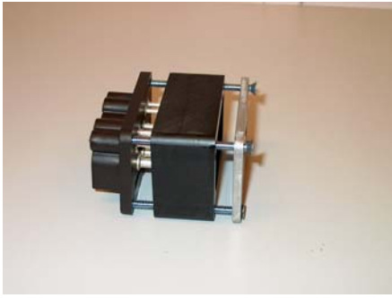
Figure 4.1 Charge Receptacle Assembly – Expanded View
