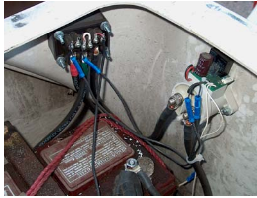
Figure 5.2 Contactor and Charge receptacle
