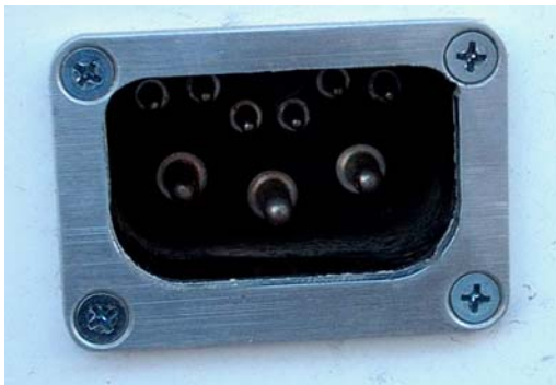
Figure 4.3 Charge Receptacle Assembly – Mounted under the Driver GEM seat
